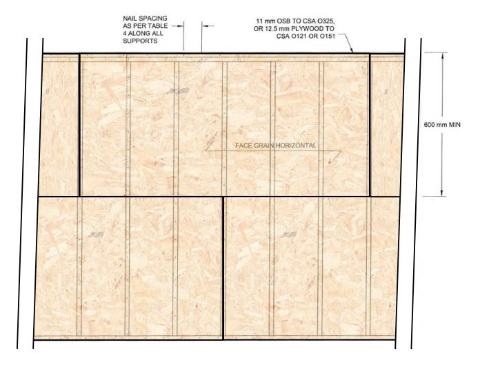
Figure A-1. Exterior sheathing and fastening for the product
