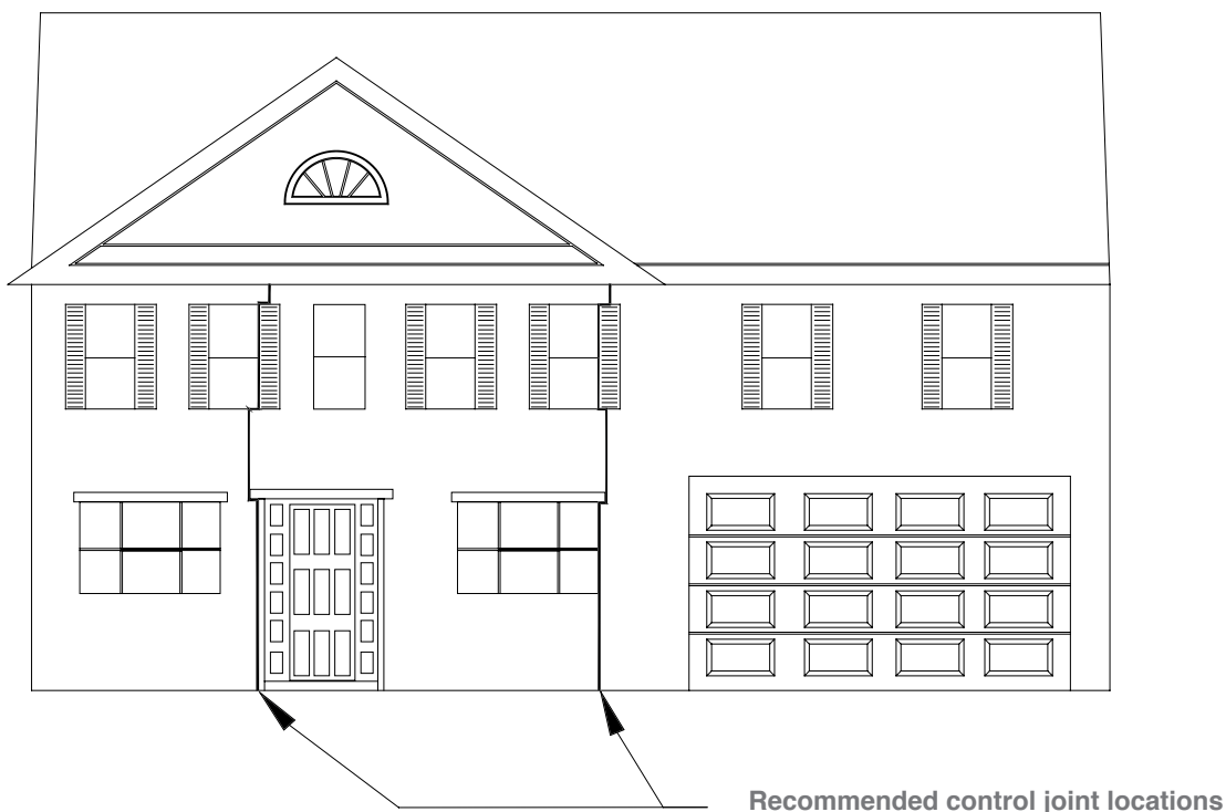
Figure 2 - Example of Residential Control Joint Placement
